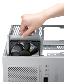
Easy-to-maintain cooling fan
